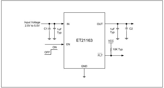
Note: Tantalum or Aluminum Electrolytic capacitors (C1 and C2) may be required for USB applications.
